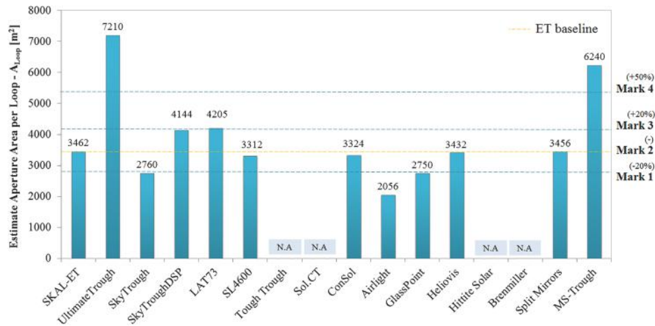
Fig. 57. Estimate aperture area per loop and evaluation marks.
