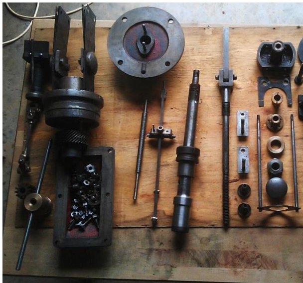
Figure 10 Single components of the governor [photo, sept. 2016]
