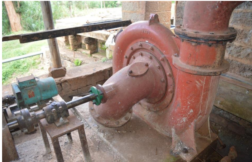
Figure 1. Francis turbine at the coffee farm [photo, July 2016]
