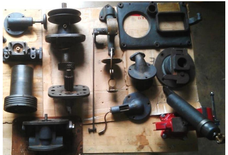
Figure 10 Single components of the governor [photo, sept. 2016]
