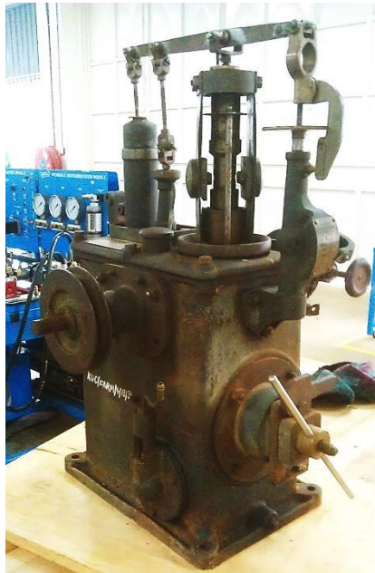
Figure 2. Gilkes & Gordon Ltd., Oil pressure governor [photo, July 2016]
