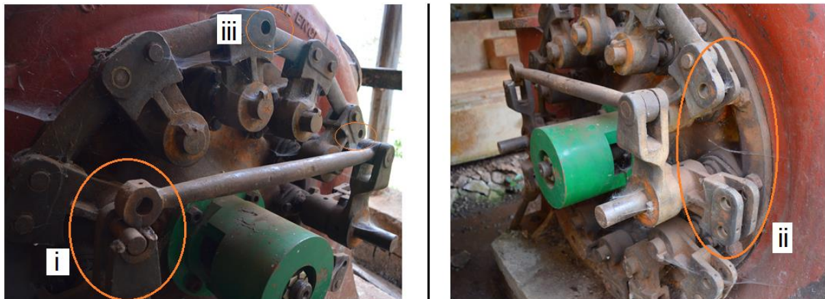
Figure 15 i-Damaged lever; ii-Missing Rods; iii-Missing pins
